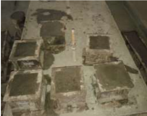
Fig . 2 Casting of cubes
